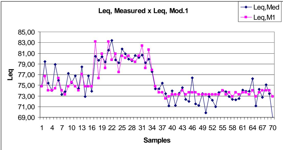
Figure 9 –Comparison between the measured and the calculated  $L_{eq}$  using Model 1.
