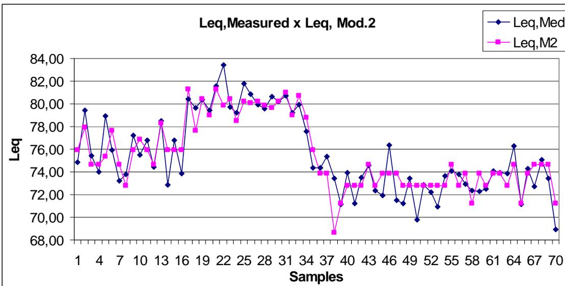
Figure 10 –Comparison between the measured and the calculated  $L_{eq}$  using Model 2.
