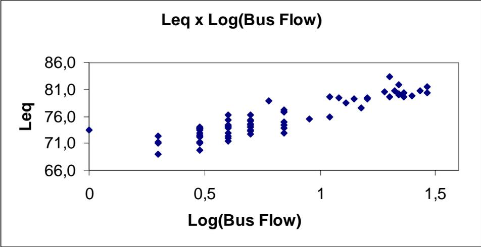
Figura 7: The variation of  $L_{eq}$  dB(A) with the logarithmic the bus flow parameter – Model 2
