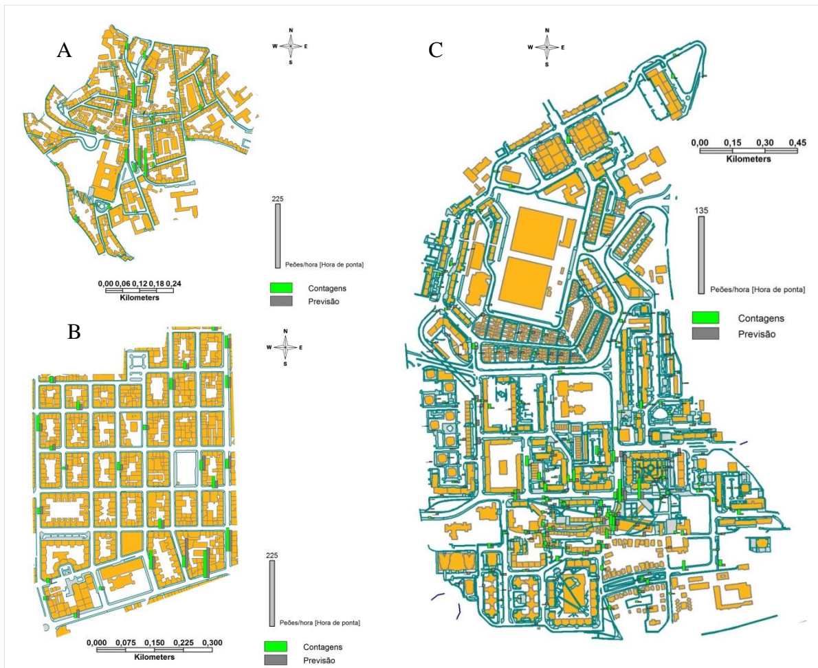
Figure 5 - Relation between the pedestrian counting and the predictions of the model for morning peak hour: (A) Graça, (B) Campo de Ourique and (C) Telheiras.
