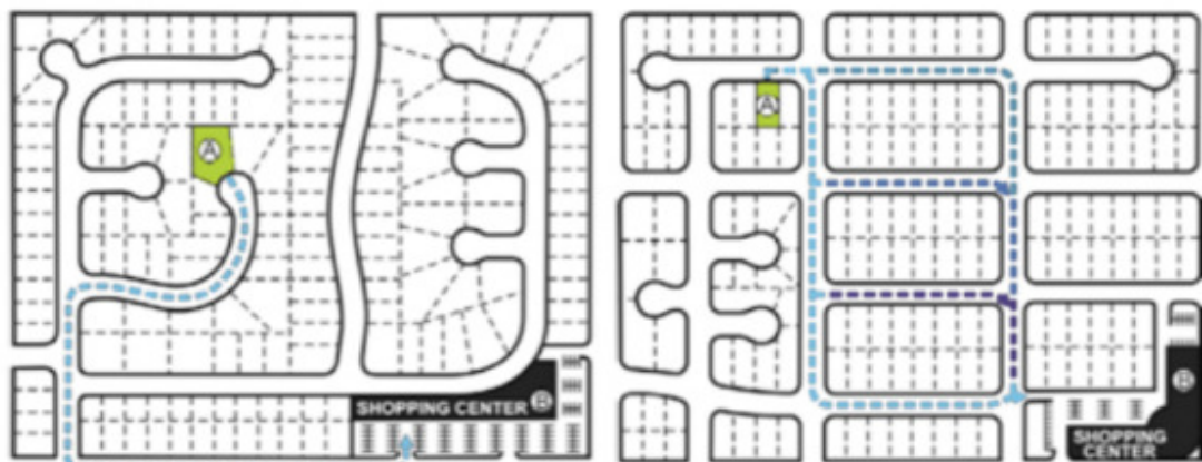
Conventional street networks (left) create longer trips and often deny choice. A network of Complete Streets (right) offers flexibility. Image: Kimley-Horn and Associates, Inc. and Digital Media Productions
